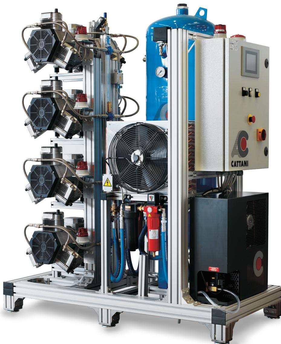
These compressors have upgraded parts which allow them to run up to 10bar, this makes it possible for the compressor to deal with the extra stresses when used with milling machines.
